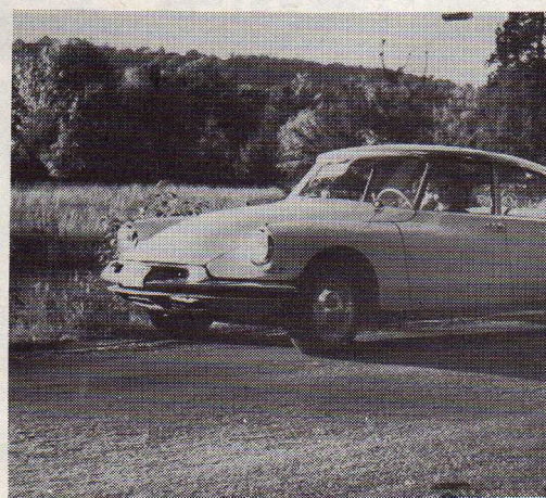
From thirteen inches above the road, car is lowered to normal driving stance.
