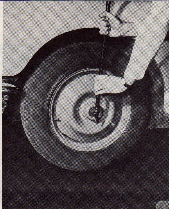
Allen type nut holds driving wheels on hexagonal drive-key. Remove with a specially supplied wrench.
