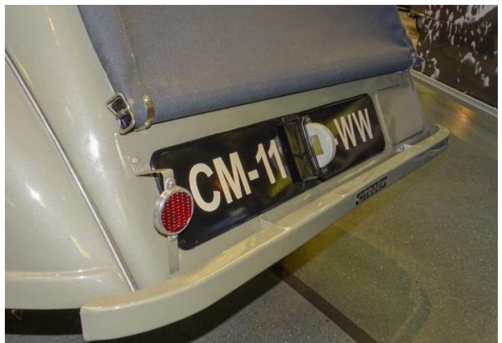
Above: 1952 2 CV shows the fabric roof and trunk covering with the small rear window. The license display area is divided in two parts, so only one lamp is required to light the registration numbers that were frequently painted directly on the car body. Below: In the early years, the 2 CV had no brake lights or turn signals. There was a single red reflector at the left, and the license lamp would have a translucent red cover.
