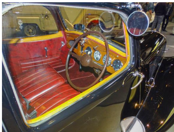
Above: Slough cars made ample use of British trim and fittings due to local content laws. Wood trim and dash holding locally sourced instruments are seen.
