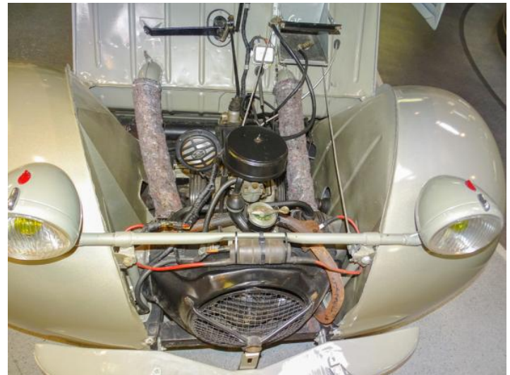
Above: 375cc air-cooled two cylinder engine hidden behind the fan, oil cooler and integral 6V generator. Ignition points, mounted on camshaft, fire a double-ended coil at center of the headlamp bar, so no distributor.
