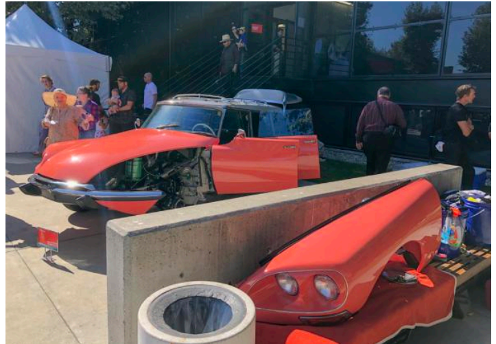
Above: Duesing's immaculate ID 21 F displays the modular body panels, front suspension details, inboard disc brakes, and unmistakable color.
