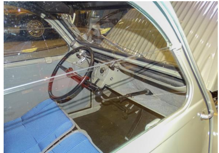
Above: The dash panel held an ammeter, but the speedometer was mounted above and left of the steering wheel under the windshield. The speedometer cable also drives the wipers so the faster one drives the faster they wipe. The split windows fold out to allow hand signals from the driver. A small grommet usually holds the windows open, but they can fall shut on unsuspecting elbows.
