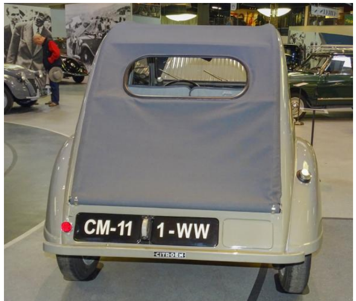
Above: 1952 2 CV shows the fabric roof and trunk covering with the small rear window. The license display area is divided in two parts, so only one lamp is required to light the registration numbers that were frequently painted directly on the car body. Below: In the early years, the 2 CV had no brake lights or turn signals. There was a single red reflector at the left, and the license lamp would have a translucent red cover.
