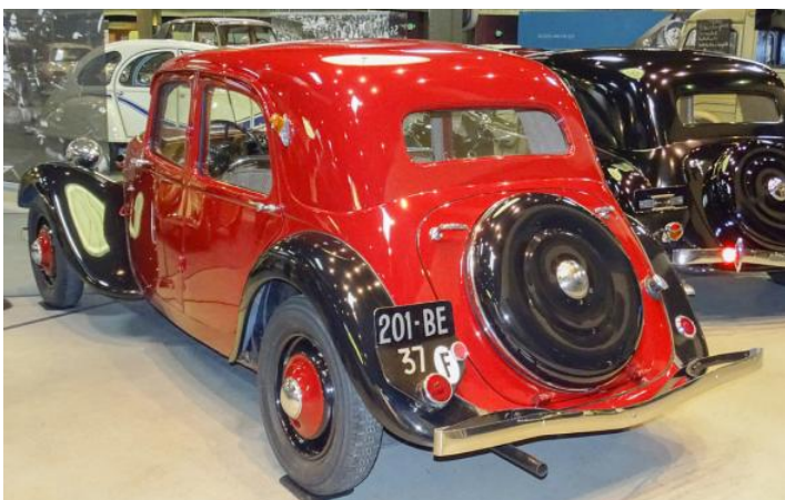
Above and Below: 1937 7C Berline, Chassis 95800, Engine 72 x 100 1628cc. All steel roof. Base models had black fenders, wheel rims, and spare tire cover, but these items could be body color for F 300 extra.
