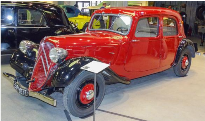
Above and Below: 1937 7C Berline, Chassis 95800, Engine 72 x 100 1628cc. All steel roof. Base models had black fenders, wheel rims, and spare tire cover, but these items could be body color for F 300 extra.
