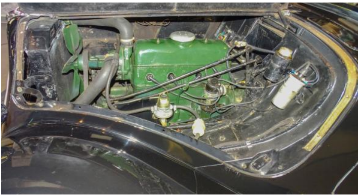
Above and Below: 1935 7C showing the uncluttered engine bay with the 1628cc unit. Rear view with the rumble seat and left hand license plate
