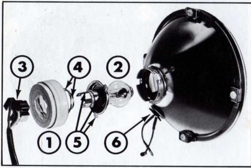
Fig. 37 - Code Route (grand  $\varnothing$ ) Lampes iode
