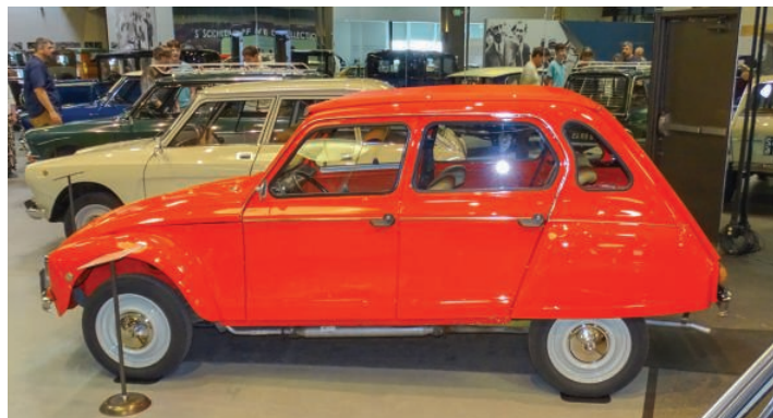
Above: The Dyane gained a third side window in 1970 well after the 2CV, and the finger grip on the door handles was inverted in 1973.
