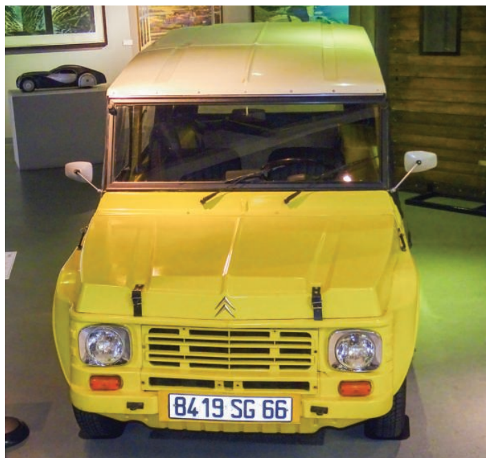
Above: The Méhari went through four versions of the front fascia design, with a fifth, unique design for the USA. This example is the newest home market version with a removable grille panel, so the whole front does not have to be lifted for maintenance.
