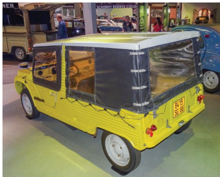
Below: Upper body could be fully enclosed, open sides or naked. Vendors like ENAC offered plastic solid panelling for the roof or sides.
