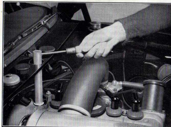
Figure 19 — Removal of the 4th sparking plug
