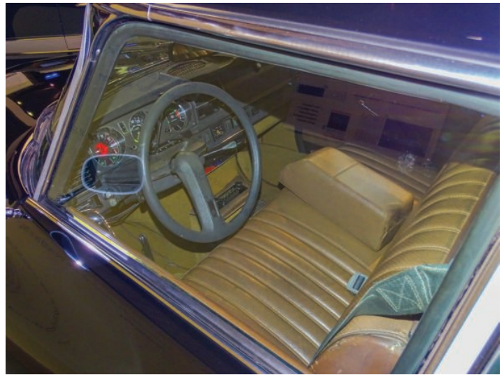
Above: Steering wheel showing the dark grey molded foam covering used from 1972 on. The dash instrument furthest left shows the blindingly bright red "STOP" lamp, center dial is speedometer, right is tachometer. Radio mounted vertically against the firewall makes reading frequency difficult.
