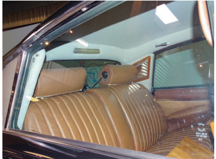
Above: DS Prestige rear compartment with reading lamps, headrests and vanity mirrors in the quarter panels. Below: clock, lighter, and controls for the rear passengers seen between the seats. Comprehensive speakers and climate control in this example.
