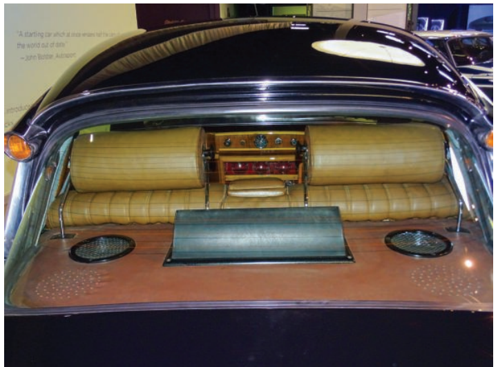
Above: DS Prestige rear compartment with reading lamps, headrests and vanity mirrors in the quarter panels. Below: clock, lighter, and controls for the rear passengers seen between the seats. Comprehensive speakers and climate control in this example.
