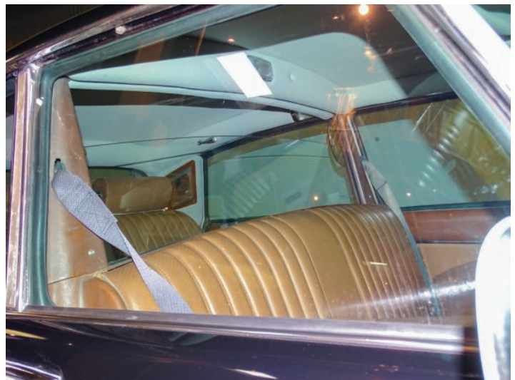
Below: DS Prestige interior division with retractable glass. Presumably the driver had to be hired to fit the car. Additional interior lamps contribute to the D model's reputation for lighting up like the sun inside.
